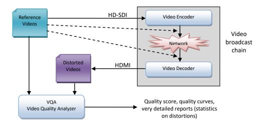
Fig. 9 – Automatic test platform organization
